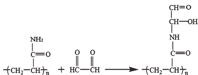
Scheme 2 Reaction between the glyoxal and amide groups on the CPAM backbone.
